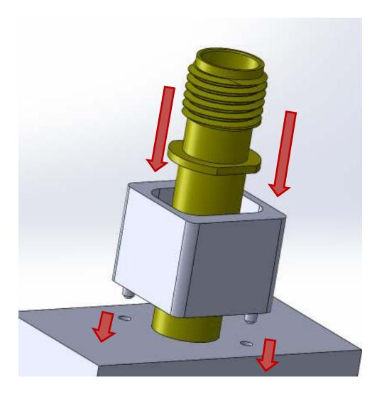
Note: Guide tool CIT-30-0 is provided with each CSP-30TS-011
