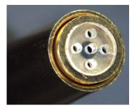
Under microscope, locate the hole in the plastic insulator
